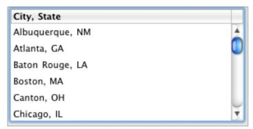
Header row text is added using **AL\_SetColumnTextProperty** with the <u>ALP\_Column\_HeaderText</u> parameter in the area's Object Method:
