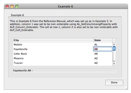
This can be controlled via the <u>ALP\_Column\_Enterable</u> property and the associated command **AL\_SetColumnLongProperty**: **AL\_SetColumnLongProperty** (eList;1;ALP\_Column\_Enterable;0) //set column 1 to be non-enterable
